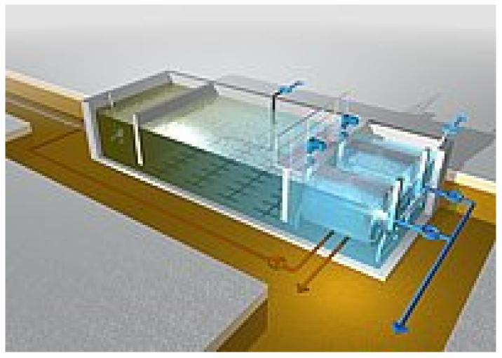
Membrane bio-reactors (MBR) are modified activated sludge systems, whereby secondary clarifiers are replaced by membrane filters.
