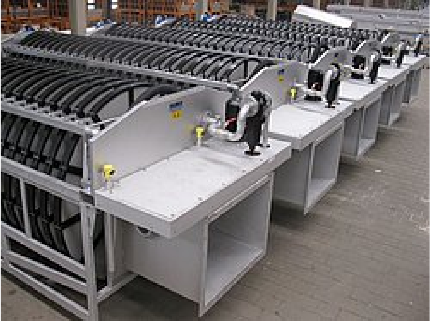
5 RoDisc® 24 screens in the factory just before delivery with the clearly visible discs consisting of individual plastic segments
