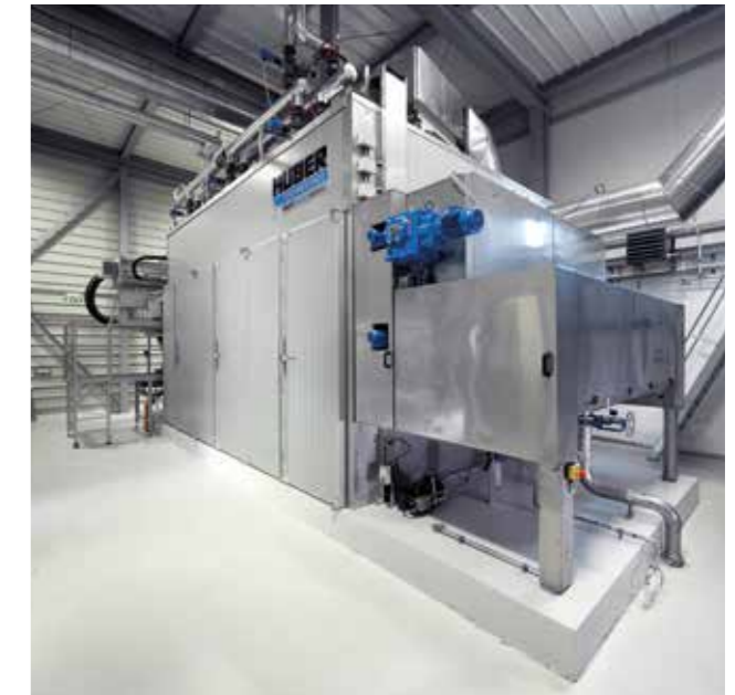
Head piece with integrated automatic belt cleaning.
