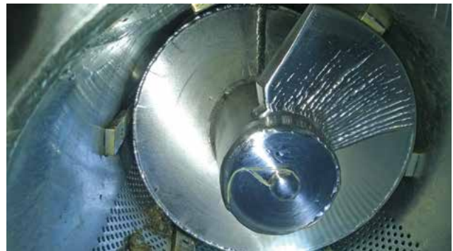
A screw shaft beginning to wear.
