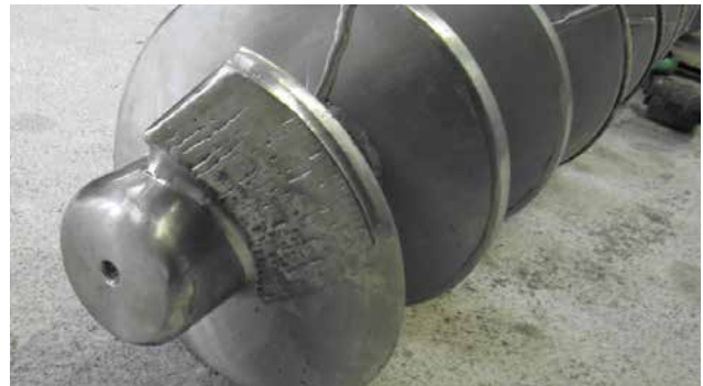
Advanced wear on a screw shaft.
