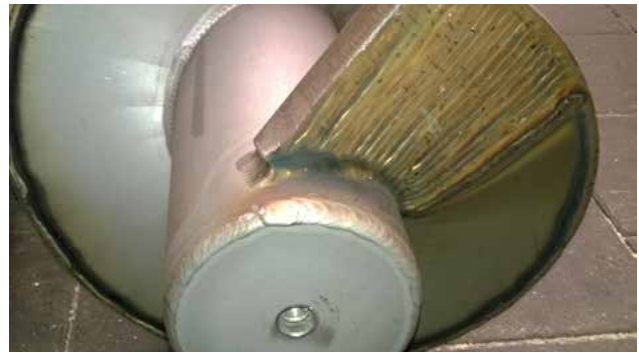
Screw shaft in new condition.
