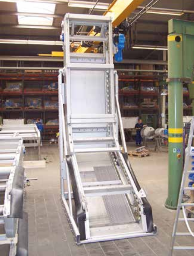
HUBER Rake-Max®-hf unit in our factory before delivery: The flat bottom section which provides favourable hydraulic conditions is clearly visible.
