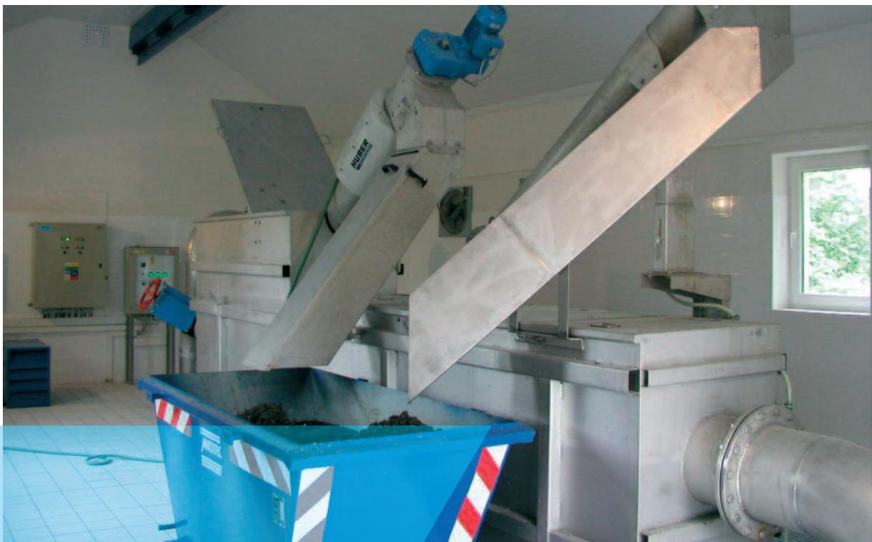
Complete Plant with integrated cross-flow lamella separator
