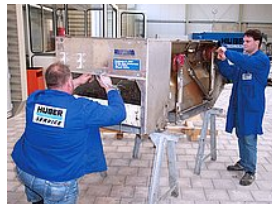
Repair and maintenance of a 3rd party step screen
