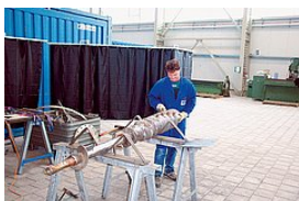
Complete overhaul of a used up worm shaft
